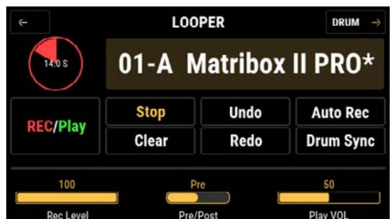
Pressing footswitch A starts recording, pressing it again starts playback, and pressing footswitch A during playback starts overdubbing:
