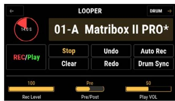
Pressing footswitch A starts recording, pressing it again starts playback, and pressing footswitch A during playback starts overdubbing:
