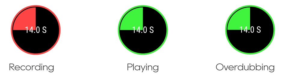
Pressing footswitch B stops recording or playback, while holding it down clears all recorded phrases.
