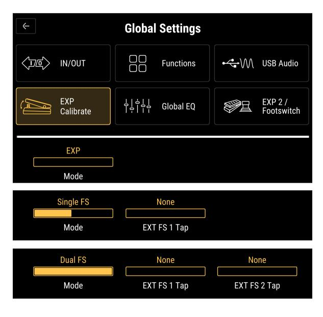
Mode: Select the type of external device to be connected to the EXP/FS jack.
