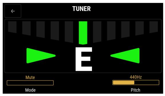
Tuner mode can be set to Mute (for silent tuning), Bypass (for dry signal through) and Thru (for effect signal through).
