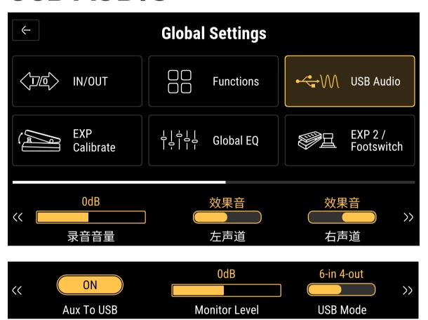
**Rec Level:** To control the master volume of the recording, ranged from -20dB to +20dB.
