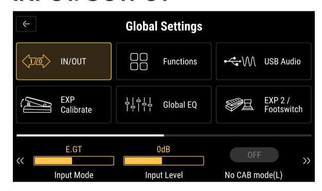
**Input Mode:** Input Mode: to adjust the impedance, including acoustic guitars (4.7M $\Omega$ ), electric guitars (1M $\Omega$ ) and line in (10k $\Omega$ ), default is E.GT.
