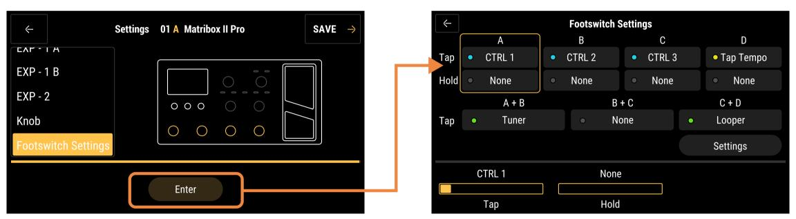
Select "Footswitch Settings" to enter, use the MENU knob or touch to directly press the Enter to locate the assigned function.
