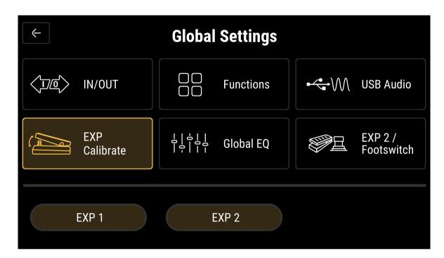
As shown, turn Quick Access Knob 1 or 2 to calibrate EXP 1 or 2.
