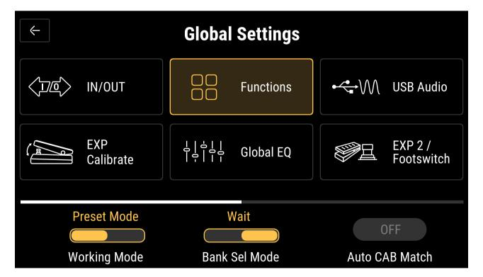
**Current Mode:** This option is used to select the footswitch function mode, which is divided into Preset mode and STOMP mode. The default mode is Preset mode. **Bank Sel Mode:** The parameters are "Wait" and "Initial". If you select "Initial", the bank will jump immediately when switching, and if you select "Wait", the bank will not jump directly when switching, but will enter the Wait Mode screen.
