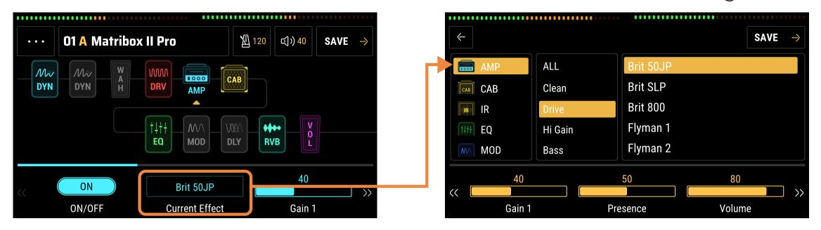
The effect details of the effect module, algorithm type and algorithm parameters can be changed in this menu.
