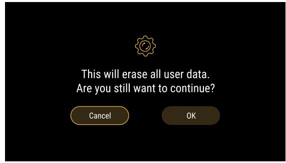
Press the PARA knob to enter the "Factory Reset" menu, then turn the PARA knob to select and click "OK" to execute the reset factory settings, which will clear all user edited presets and personalized settings and reset the device to the factory state.
